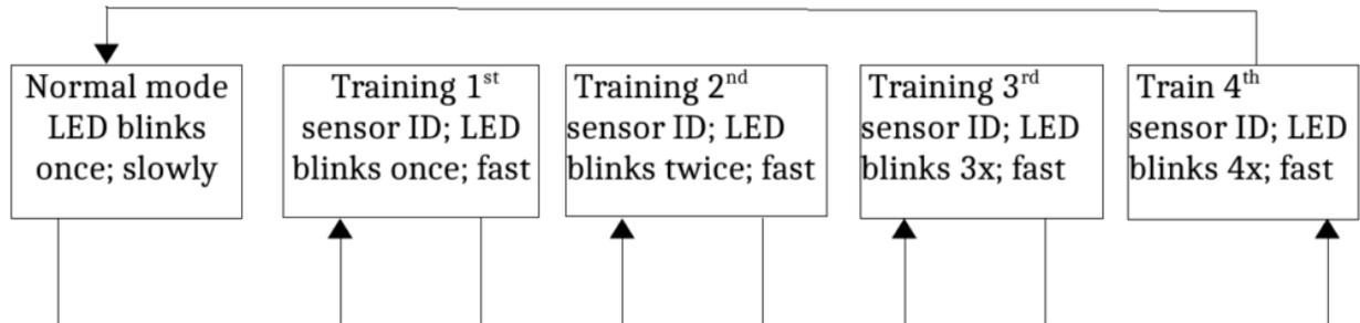
Further down below are the unit's operating modes. Going from one mode to the other is done sequentially as the arrows depict and it is accomplished by pressing the small black button. Do allow **at least 4 seconds** between presses of the button:
